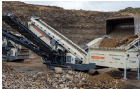
Large feed box allows closed circuit process.
